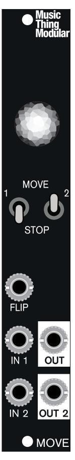
Switches determine how the two channels respond.
