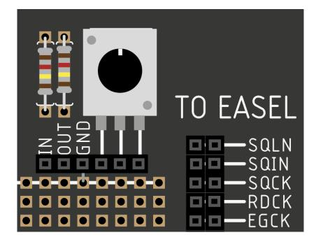
2. You then need a range of resistors to patch between signals: Add two vertical rows of female headers with four empty holes between them. Then solder resistors between the rows, connecting with the headers beneath the board
