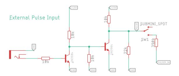
I do this using two NPN transistors—I've used 2N3904 or 2N2222 plus six resistors.
